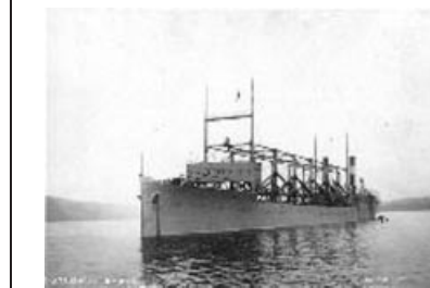
Figure 7. USS Cyclops (1910–1918) anchored in the Hudson River on October 3, 1911. U.S. Navy Photo. General characteristics: Class and type: Proteus-class collier; displacement: 19,360 tons full; length: 542 ft; beam: 65 ft; draft: 27 ft 8 in; speed: 15 knots (17 mph); complement: 236 officers and enlisted; Armament: 4 × 4 in guns. The USS Cyclops was lost at sea in the “Bermuda Triangle” in 1918 with all 306 crew and passengers without a trace. Courtesy of the US Navy.
